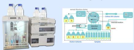
A special feature of LC-03 is that the SPE column can be washed from two directions. It is very efficient to remove trapped particles by washing the SPE column in the reverse direction. It also helps to obtain good peak shape for very retentive compounds. Thanks to this feature, one SPE column can be used for at least 50 samples and in most cases the sample does not need filtration. Below are two examples. The left is for benzopyrene and the right is for caffeine.
